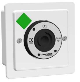
The construction of PMGS' Zeus SP is of machined brass and injection moulded polymer with stainless steel Teflon<sup>™</sup> coated rolling pins. Each of the gas specific components have the gas service placed onto it to ensure safety and compliance with the standard. The wall mounted terminal units incorporate an anti-swivel pin to prevent rotation of installed equipment.
