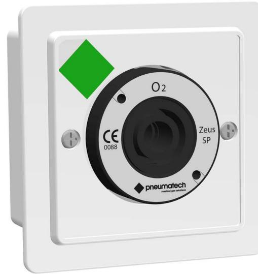
The construction of PMGS' Zeus SP is of machined brass and injection moulded polymer with stainless steel Teflon™ coated rolling pins. Each of the gas specific components have the gas service placed onto it to ensure safety and compliance with the standard. The wall mounted terminal units incorporate an anti-swivel pin to prevent rotation of installed equipment.
